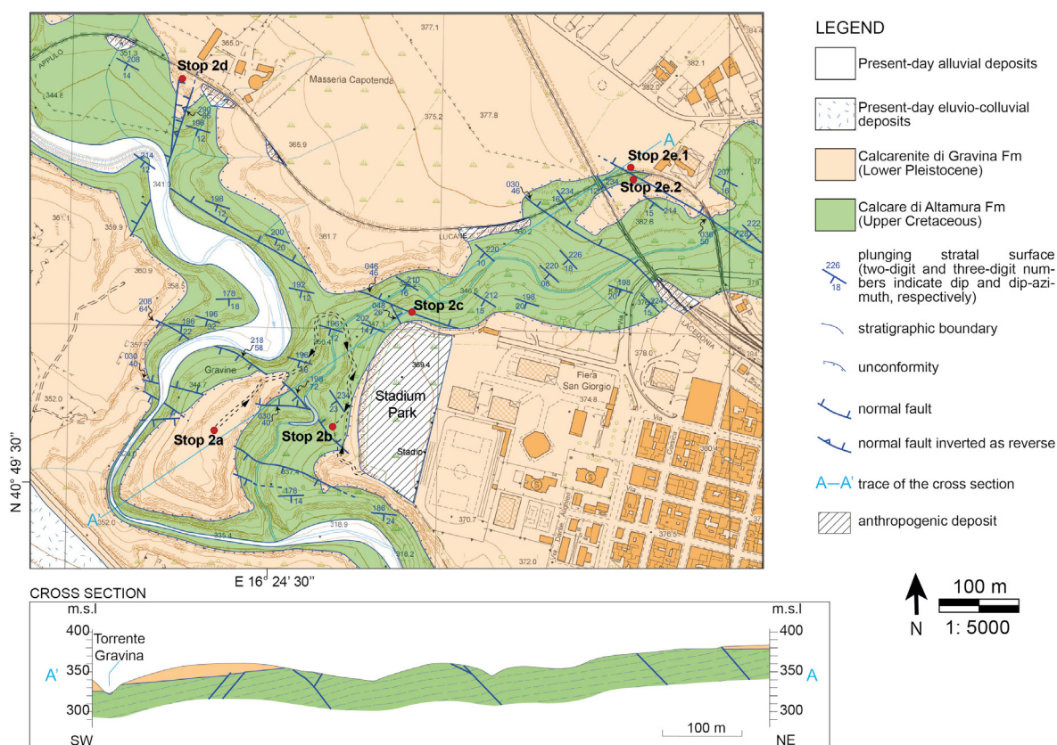
Fig. 17 - Geological map and related cross section of the northern part of the "Gravina di Gravina" canyon, surveyed at 1: 5,000 scale. See location in Fig. 16.
