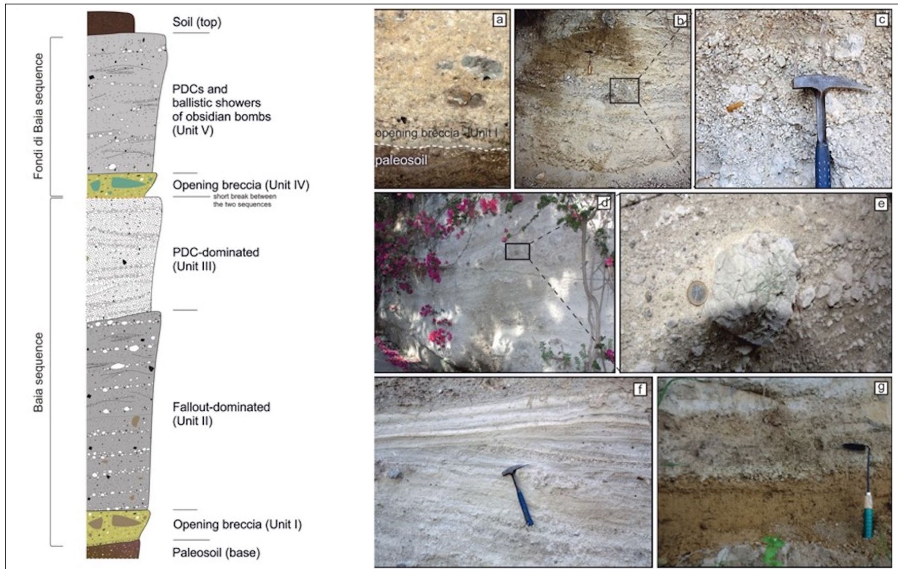
Fig. 18 - Left: composite stratigraphic succession of Baia and Fondi di Baia eruptions. Right: pictures of the Baia succession. (a) Opening breccia (Unit I) which overlies the basal paleosol. (b) Fallout and PDC deposits of Unit II. (c) Detail of a pumice layer shown in (b). (d) PDC layers of the upper part of Unit II. (e) Detail of a breadcrust bomb shown in (d). (f) Cross-bedding of surge deposits of Unit III. (g) Pumice fallout deposit of Unit II overlying a paleosol 20 km north of the vent. On the left, idealized composite stratigraphy of the different phases of the eruption. Modified after Pistolesi et al. (2017).
