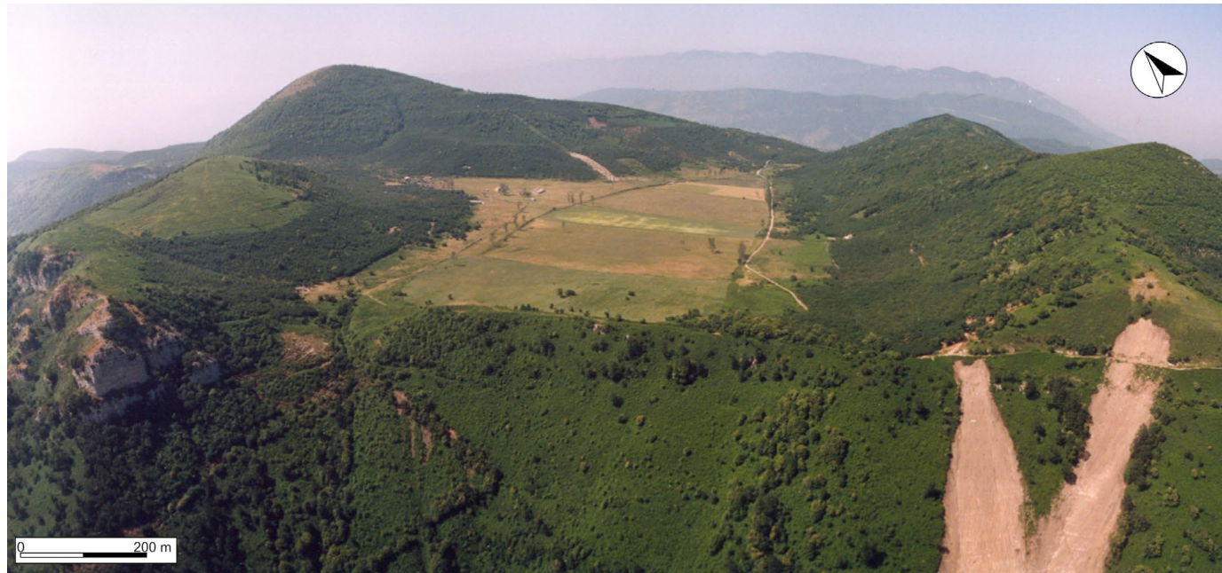
Fig. 25 - Piani di Prata polje at the top of the Pizzo D'Alvano limestone belt, with the detachment area of two May 1998 landslides in an oblique aerial view taken slightly after the 1998 event.
